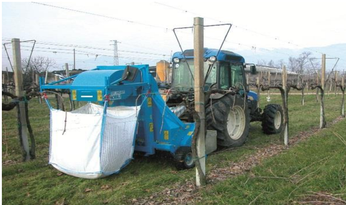
Figure 6. Mulcher for the collection of pruning residues (source: https://www.nobili.com/trp-rt-rtt/s9caf9640 )
